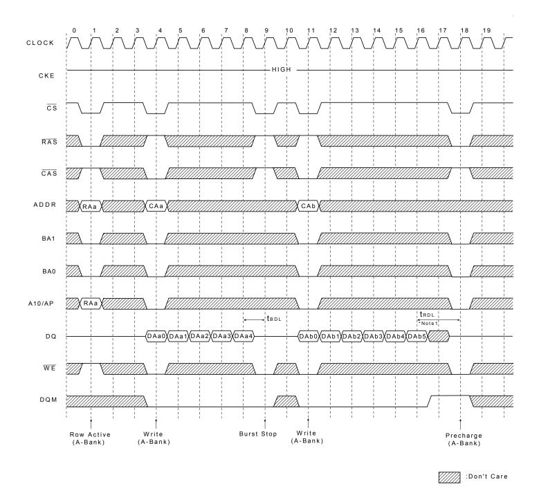
\*Note: 1. Data-in at the cycle of interrupted by precharge can not be written into the corresponding memory cell. It is defined by AC parameter of tRDL. DQM at write interrupted by precharge command is needed to prevent invalid write.
