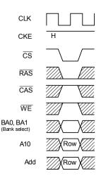
Fig. 2 Row address stroble and bank active command
