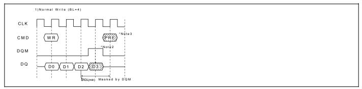
\*Note: 1. To prevent bus contention, DQM should be issued which makes at least one gap between data in and data out. 2. To inhibit invalid write, DQM should be issued.
