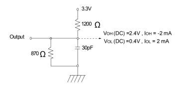
(Fig. 1) DC Output Load Circuit
