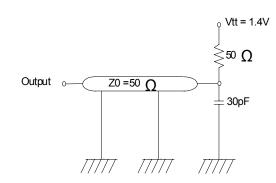
(Fig. 2) AC Output Load Circuit
