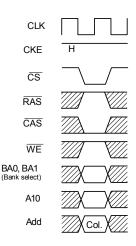
Fig. 5 Column address and read command
