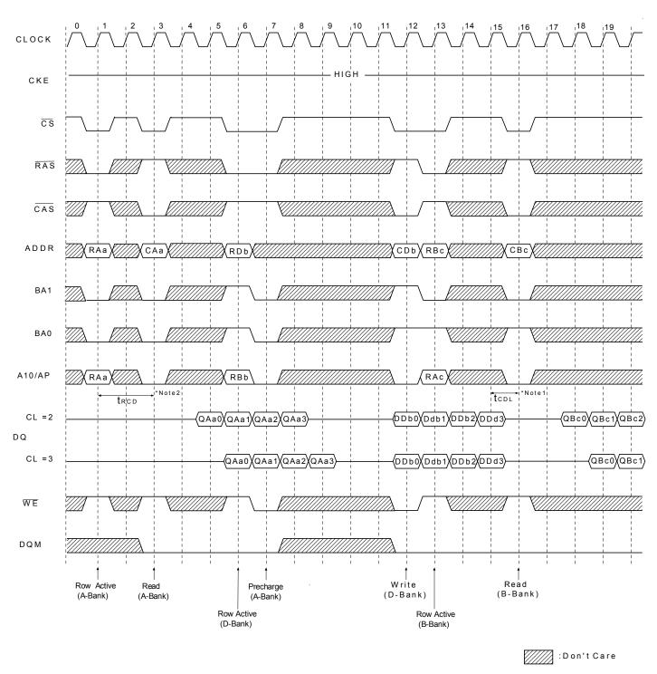
Read & Write Cycle at Different Bank @ Burst Length = 4
