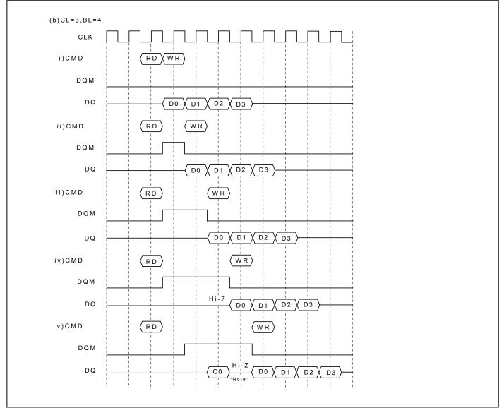
\*Note: 1. To prevent bus contention, there should be at least one gap between data in and data out.
