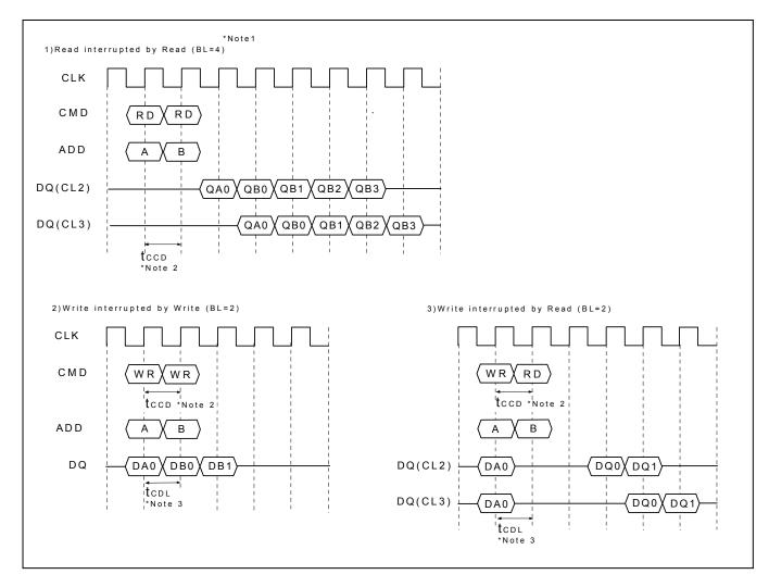
\*Note: 1. By "interrupt" is meant to stop burst read/write by external before the end of burst. By " $\overline{CAS}$  interrupt", to stop burst read/write by  $\overline{CAS}$  access ; read and write.
