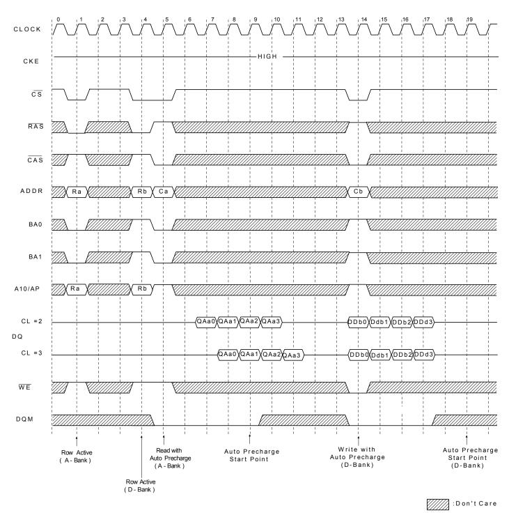
\*Note: 1. tcpL should be controlled to meet minimum tras before internal precharge start. (In the case of Burst Length = 1 & 2)
