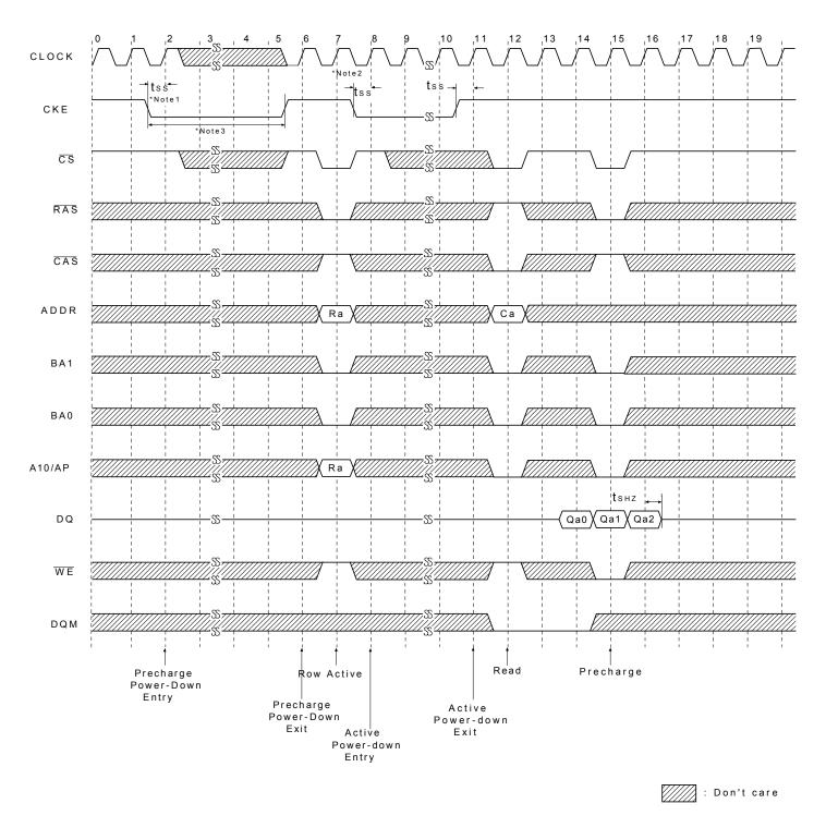
\*Note: 1. All banks should be in idle state prior to entering precharge power down mode. 2. CKE should be set high at least 1CLK + tss prior to Row active command.
